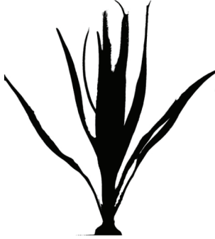
Fig. 4 Illustration of the projected area of a vegetation element used to compute the frontal area A_f (black color)
