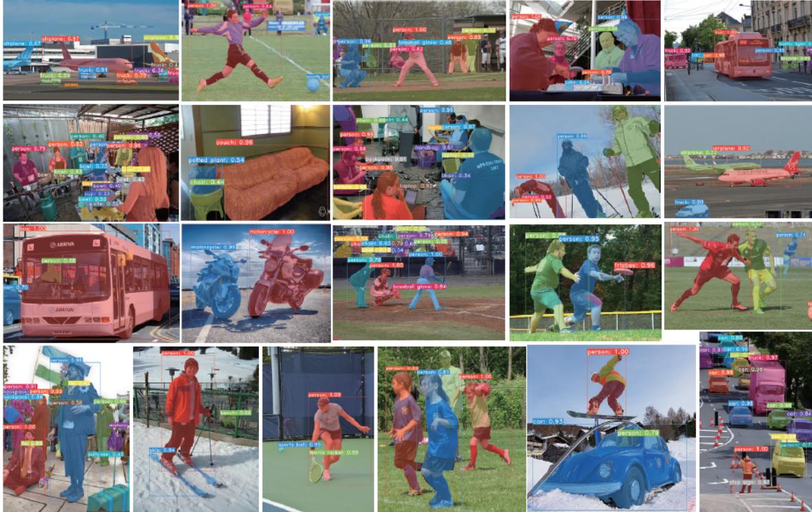
Figure 6: YOLACT evaluation results on COCO’s test-dev set. This base model achieves 29.8 mAP at 33.0 fps. All images have the confidence threshold set to 0.3.
