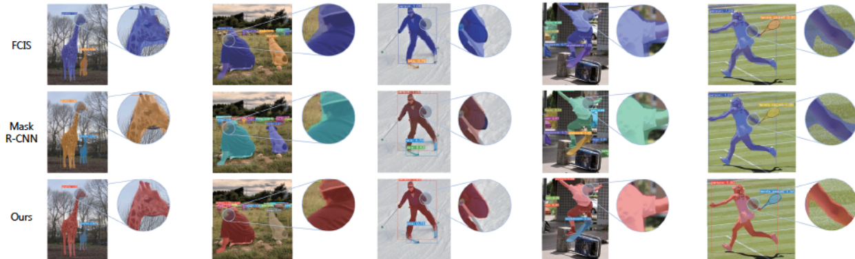
Figure 7: Mask Quality Our masks are typically higher quality than those of Mask R-CNN [18] and FCIS [24] because of the larger mask size and lack of feature pooling.
