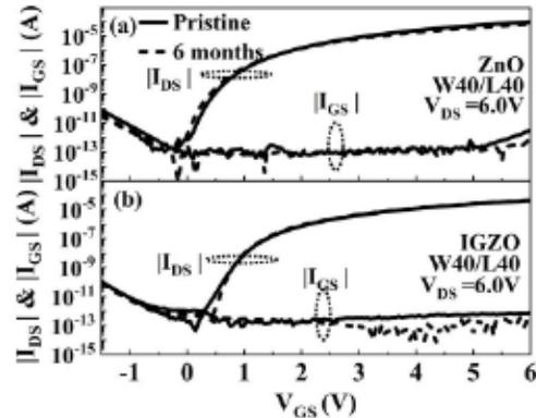
Fig. 7. Representative transfer characteristics comparison of pristine and 6 months after fabrication for (a) ZnO and (b) IGZO TFTs.
