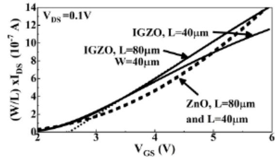
Fig. 4. Comparison of normalized  $I_{DS}$  versus  $V_{GS}$  at  $V_{DS} = 0.1$  V for ZnO and IGZO at different channel lengths.
