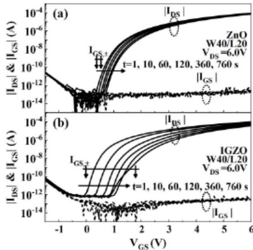
Fig. 5. Comparison of the representative transfer characteristic after the gate and drain bias stress cycles for (a) ZnO and (b) IGZO.
