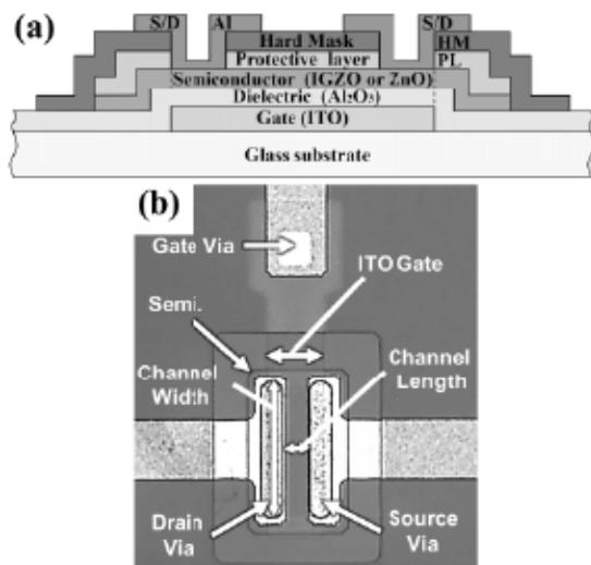
Fig. 1. (a) Cross section of a TFT. (b) Top view of a TFT with  $W = 40 \mu\text{m}$  and  $L = 20 \mu\text{m}$ . The S/D vias are  $5 \mu\text{m}$  wide with S-D metal overlap of  $2.5 \mu\text{m}$  for alignment tolerance.
