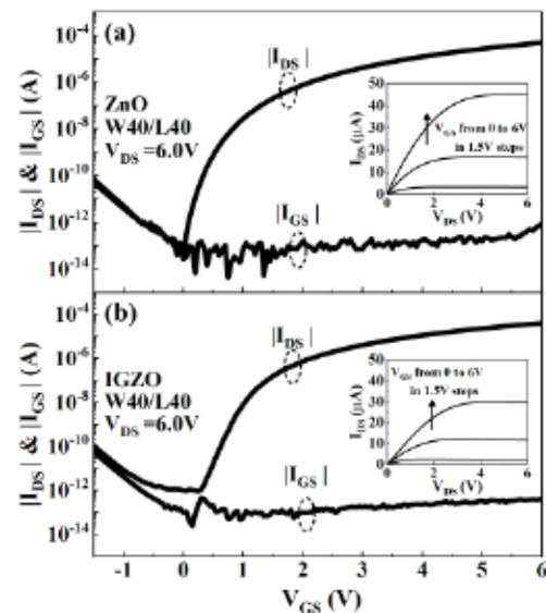
Fig. 2. Representative transfer characteristics for (a) ZnO- and (b) IGZO-based TFTs, respectively. Inset:  $I_{D}-V_{D}$  output characteristics for the respective TFT.
