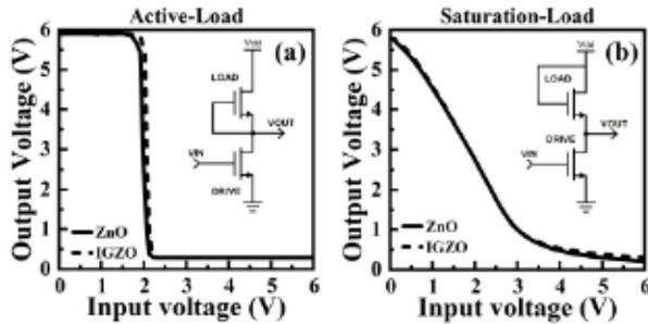
Fig. 8. DC response for logic inverters with (a) active load and (b) saturation load, respectively.
