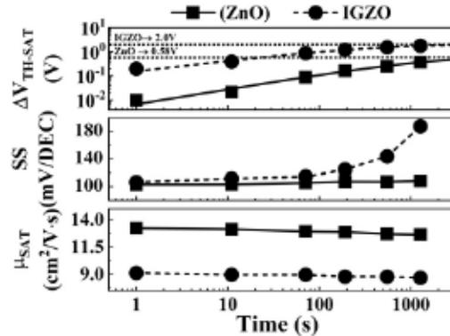
Fig. 6. Extracted saturation threshold voltage shift ( $\Delta V_{TH-SAT}$ ), SS, and saturation mobility as a function of the stress time.
