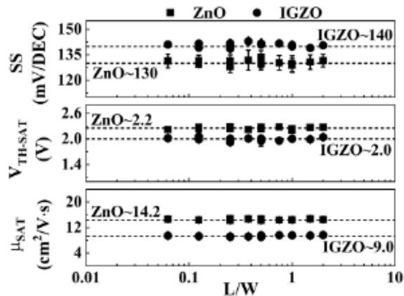
Fig. 3. Extracted saturation mobility, saturation threshold voltage, and SS as a function of the device aspect ratio. Dashed lines represent the average value. The horizontal trend suggests devices behaving normally with negligible parasitic effects.
