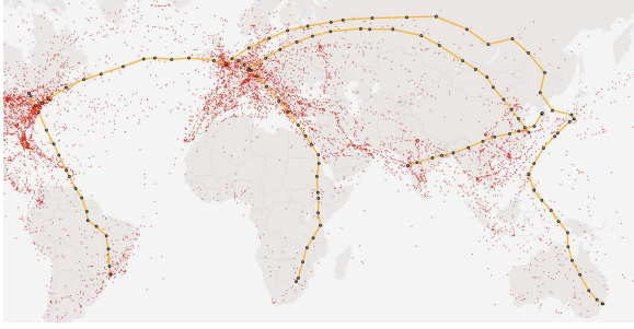
Figure 5: Using in-flight airplanes as network hops. This snapshot from July 11, 13:49 UTC shows 11,082 in-flight airplanes as well as the paths between a few major cities through them.
