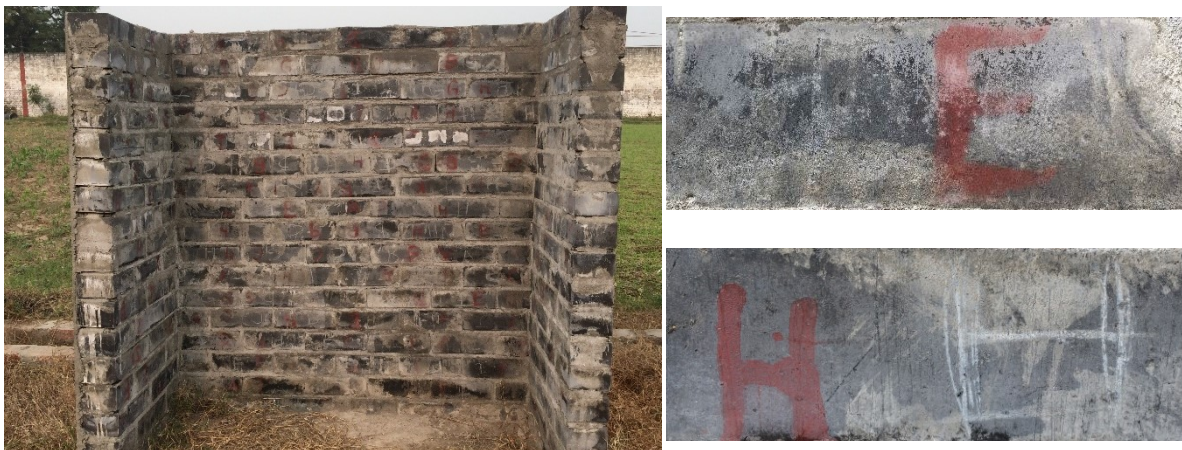
Figure 7. A brick wall prototype (left) and two bricks (right) made of 1M NaOH-activated biomass ash binder (Note: The wall was built in Muzaffarnagar, India in July 2017)
