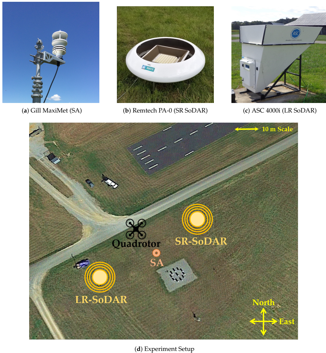
Figure 4. (a) The Gill MaxiMet sonic anemometer used to measure wind velocity 10 m AGL. (b) The Remtech PA-0 sensor (SR SoDAR) used to measure wind velocity from 10 to 120 m AGL. (c) The ASC 4000i sensor (LR SoDAR) used to measure wind velocity from 30 to 120 m AGL. (d) The experiment setup used to validate quadrotor wind estimates from 10 to 120 m AGL.
