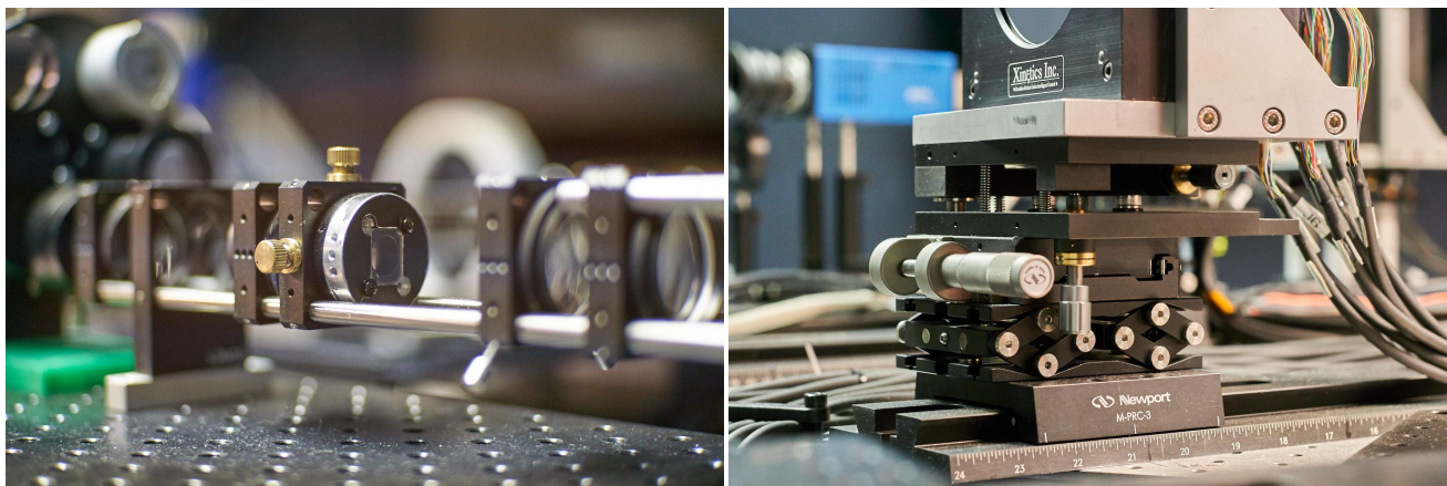
Figure 3: The microlens mounted in a x - y translation stage (left) and one of the high-altitude DMs mounted on a jack and on a linear stage (right).
