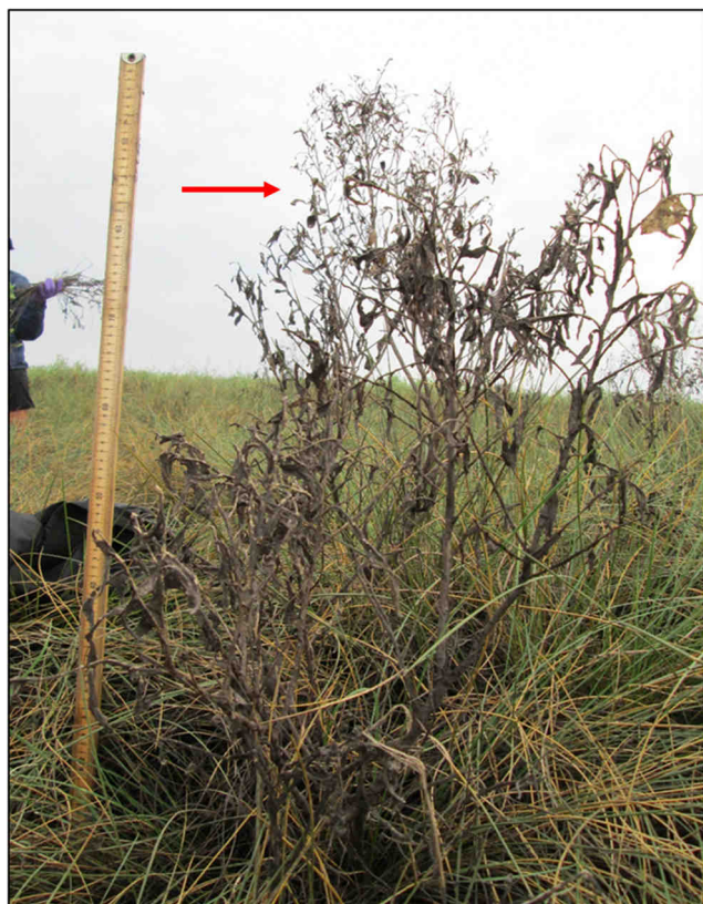
Fig. 4 Mud and wrack caught on the plants showing the maximum height (red arrow by the meter stick: \sim 0.85 m) of the flood water near core 20
