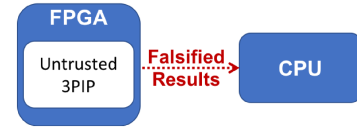
Fig. 1. Threat model considered in this paper: The untrusted 3PIP in the FPGA sends falsified results to the CPU.
