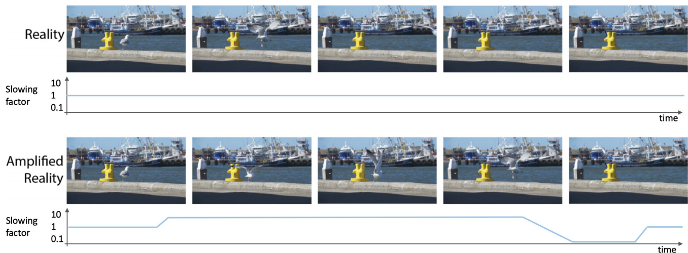
Figure 1: Altering the speed of reality allows us to observe fast events in great detail. With amplified vision, the take-off of the seagull is visible in slow-motion. The relative speed of slow-motion is first low and then accelerating to catch up with reality.
