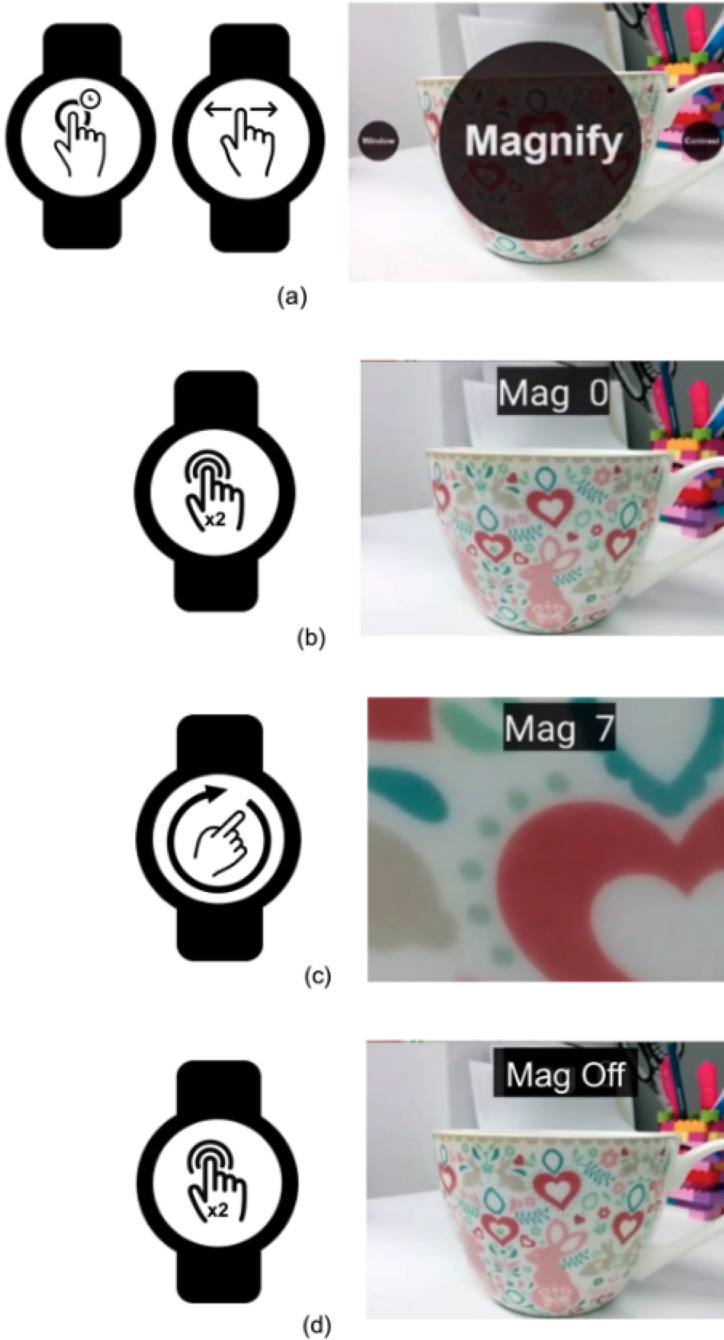
Fig. 8. Interaction Flow of ForeSee (the images on the right column are the screen shot images a user can see through ForeSee in each interaction step, and the smartwatch figures on the left column represent the gestures to trigger a corresponding step): (a) Long press to trigger the menu and swipe to the left or right to switch to a specific enhancement method; (b) Double tap to select an enhancement; (c) Clockwise or counterclockwise slide to adjust the enhancement level; (d) Double tap to turn off/on the enhancement.
