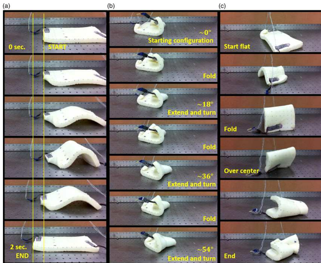
Fig. 12. Left: The robot demonstrating a crawling gait. This gait produces a forward locomotion speed of \sim 13 mm/s. Center: The robot demonstrating a turning gait. Each motion of this configuration produces \sim 18^\circ of rotation. Right: The robot demonstrating a flipping behavior.
