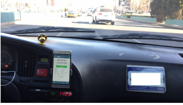
Fig. 6. We evaluate our system with a city scale deployment on taxi-based testbed. An Android App, GPS Logger [63], is used to collect real-time trajectories of taxis.
