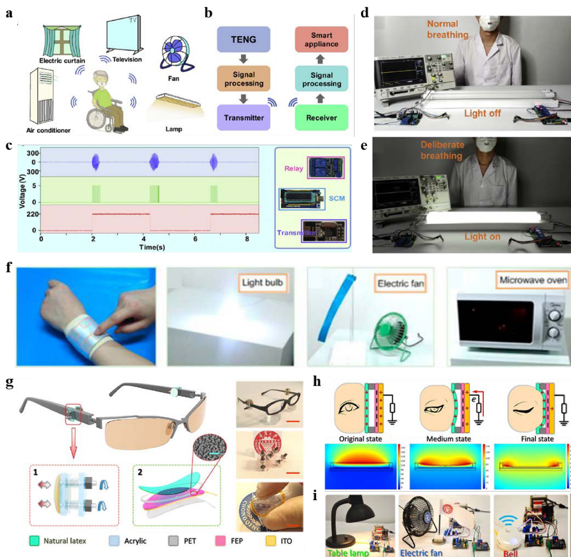
Figure 9. Control of household objects. a) Schematic illustrating household object control. b) Signal transmission and processing flow of the breathing operated HMI. c) Graph on the left shows the signals from the TENG (top), the switched square signal (middle), and electrical power (bottom). Right frame shows the electronics for signal processing and transmission including the relay, single-chip microcomputer (SCM), and transmitter. d) Normal breathing while the subject wore the TENG device on a mask did not turn on the light. e) Deliberate breathing turned on the light. f) Washable electronic textile (WET) mounted on the wrist (left) and control of home appliances (right frames). Reproduced with permission. [178] Copyright 2018, American Chemical Society. g) Eye-triggered mechanosensor on the frame of glasses.
