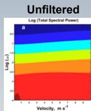
The temporal filtering introduces oscillations while suppressing the power at higher frequencies thus in part counteracting the effects of advection.
