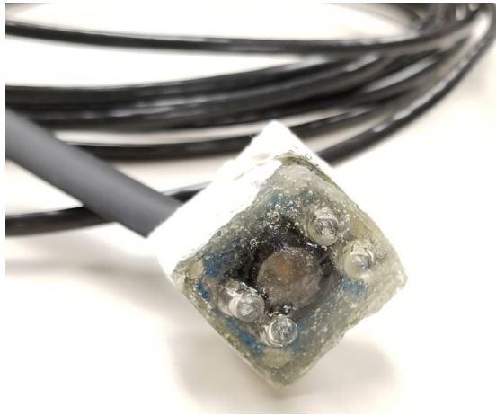
Fig. 4. Epoxy potted turbidity sensor.
