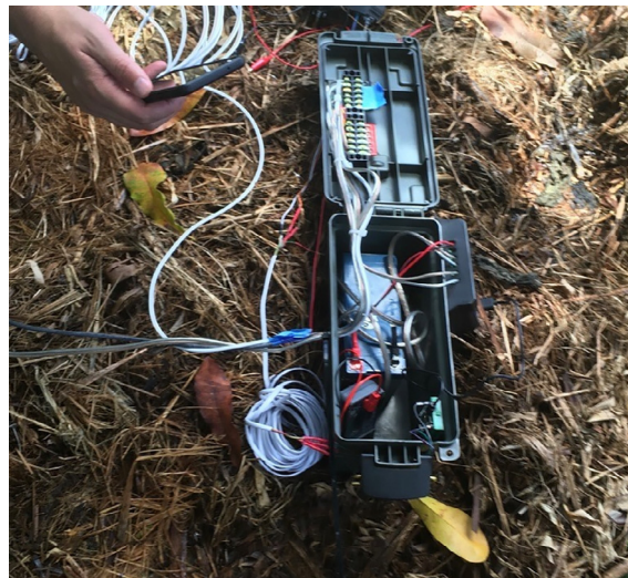
Fig. 1. .Assembled ammo-can battery box deployed in Hilo, Hawai'i. Shown with lid open.
