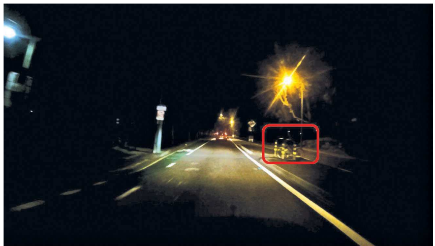
FIG6 Reliably detecting and recognizing VRUs, such as cyclists, is difficult enough under normal conditions but is compounded in poor visual conditions and when the VRU (indicated by the red box) is partially obscured by other objects in the environment.
