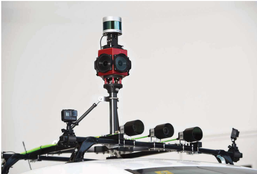
FIG1 A typical sensor suite on top of a car, with multiple cameras and lidar sensors. (Source: QUT; used with permission.)
