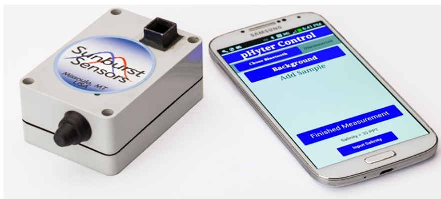
FIGURE 3 | Sunburst pHyter, a hand-held pH meter, with controlling mobile app (courtesy by Dr. M. DeGrandpre, University of Montana, United States).
