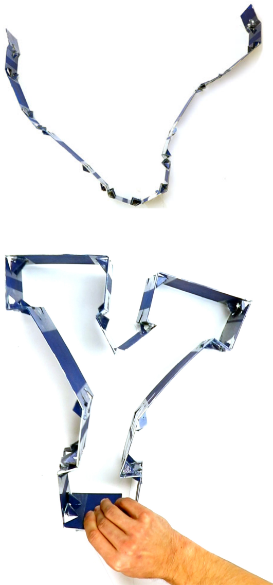
FIGURE 9. BYU block Y designed using the P-STHS model in its open and closed positions. The shape is closed by pulling on a wire passing through each strip. The images are scaled to fit the page.
