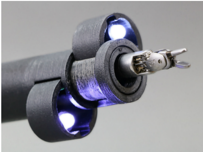
Figure 11: Multiplying Cylinders mechanism with ISI forceps inserted. LED lights included to demonstrate potential application as a dual-source flashlight or a vehicle for stereoscopic vision cameras.
