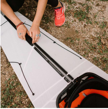
FIGURE 3: An origami kayak. The retaining channel being installed is one of several techniques that create stability. Others not shown include bulkheads and straps. (Image used with permission from Oru Kayaks™, downloaded from www.orukayak.com )
