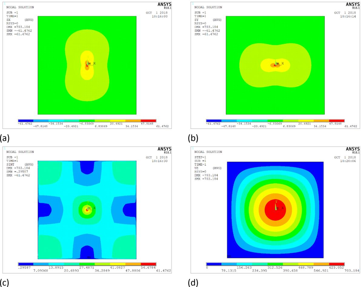
Figure 3 Simulation result of rectangular plate model (a) X-direction strain, (b) Y-direction strain, (c) strain intensity, (d) Z-direction displacement.
