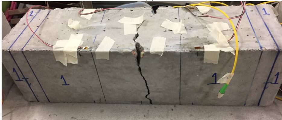
Fig. 9 Comparison of detected crack compared with reference crack (a) and photo of after cracking (b) for Sample 1
