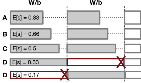
Fig. 5. Parallel job using BSP on transient servers with backup replica tasks where k = 4 and r = 1 .
