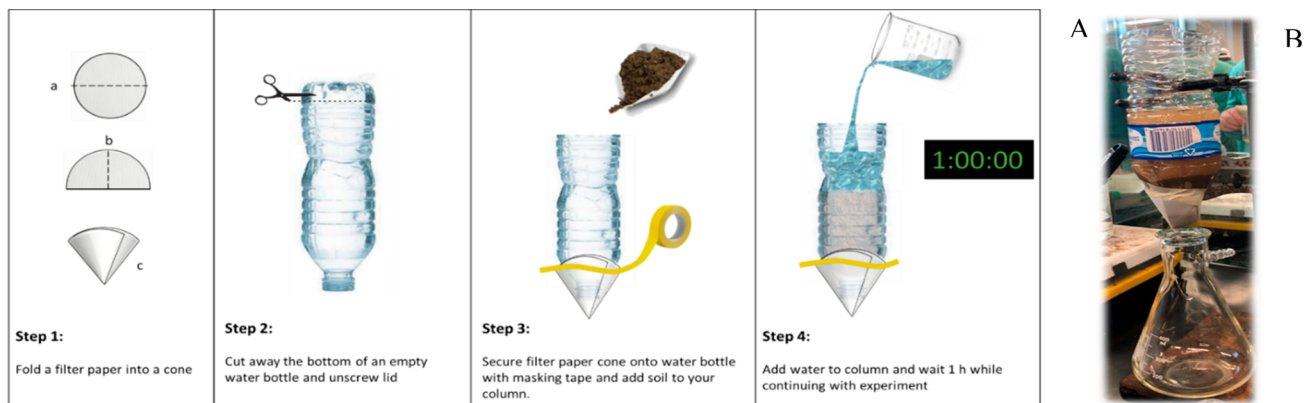
Figure 4. (A) Step by step procedure for constructing the soil column from the used water bottle; (B) the prepared soil water column.
