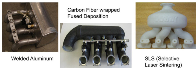
Figure 4. DF 1.2.1.1 attribute with respect to materials and manufacturing method (DP 1.2.1.1.2).
