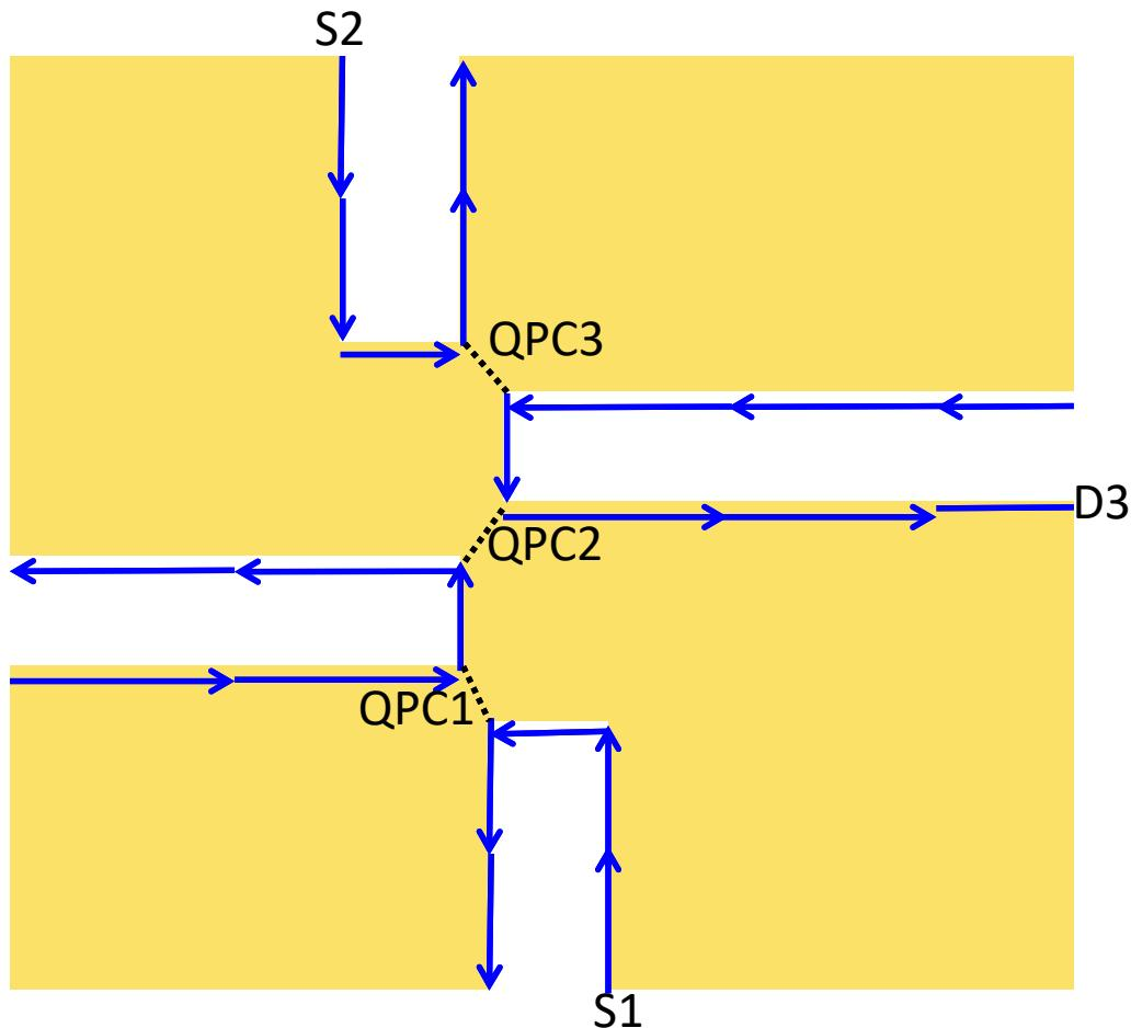
Fig. 1. Schematics of anyon collider. Quantum Hall liquid is colored yellow. Dotted lines represent anyon tunneling. Arrows show the charge propagation directions along the edges.
