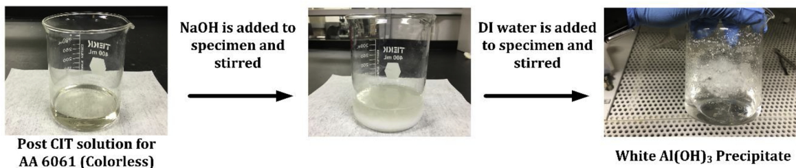
Fig. 7. Chemical analysis to show the etching effect by adding NaOH and DI water. (a) chemical analysis of silane solution before CIT showing no precipitate, and (b) chemical analysis of post CIT process solution showing white \text{Al}(\text{OH})_3 precipitate.
