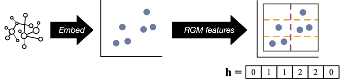
Fig. 1: Overview of our framework. Given an input graph, node representations are learned via an appropriate embedding technique (§ II-B). Our proposed feature mapping RGM then aggregates the graph’s node embeddings in vector space (§ III).
