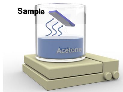
Figure 2 Removing PMMA by acetone vapor.
