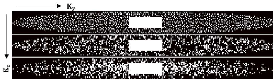
Supporting Figure S2: Three 2D undersampling patterns were tested: Poisson disc (top), uniform-density random (middle) and variable-density random (bottom) with 4-fold acceleration.
