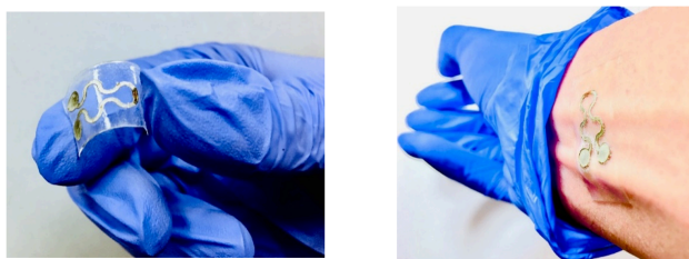
Figure 2. Optical images of the gas sensor (left) bent over a cylinder with a radius of 5.53 mm and (right) attached to the back surface of the hand.
