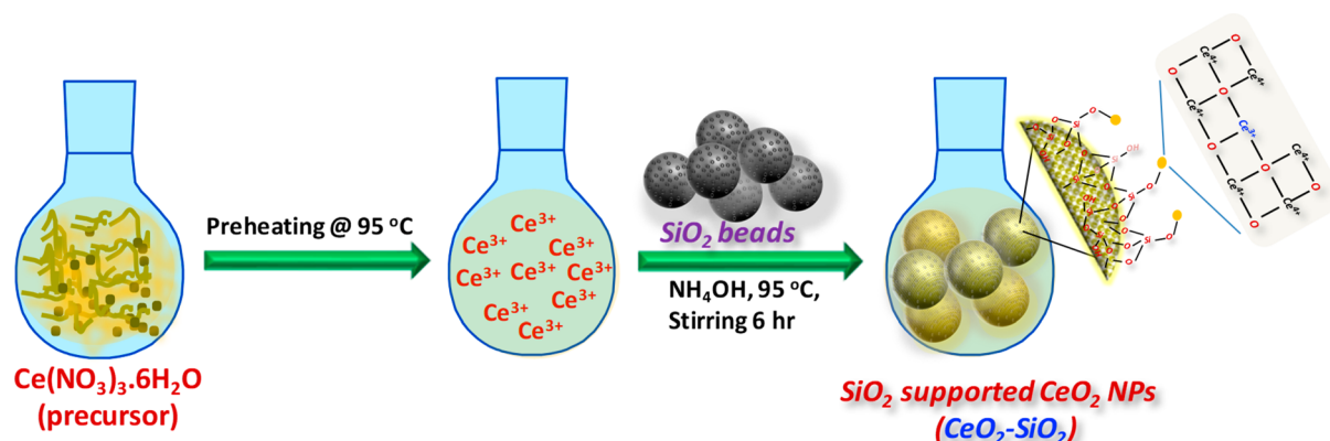
Scheme 1. Schematic Representing the Functionalization of SiO 2 with CeO 2 NPs
