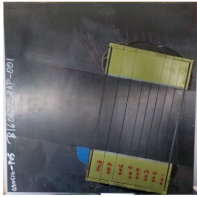
Fig. 4. UD CFRP plaque (approximately 300 mm x 300 mm) with fibers oriented in the vertical direction, and the tabbed specimens after waterjet cutting.
