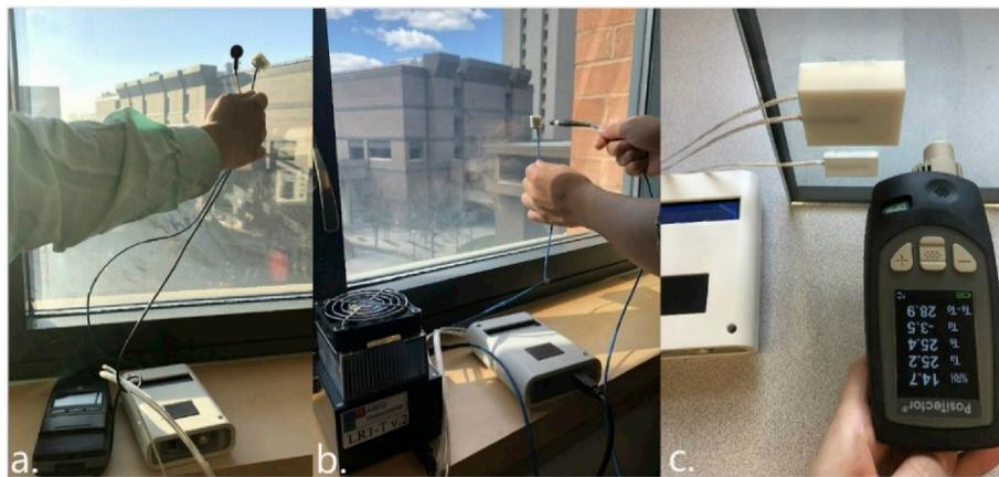
Fig. 7. a. luminosity sensor's illuminance calibration using KMT-10MA; b. Luminosity sensor's illuminance calibration using ASEQ LR1-T v.2; c. Surface temperature sensor calibration using PosiTector.
