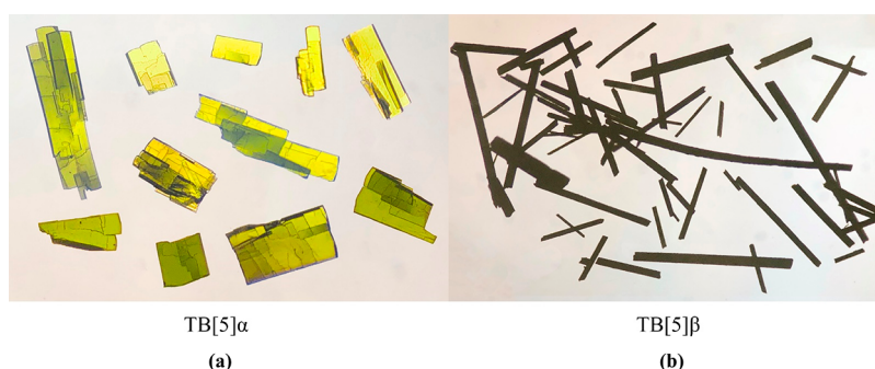
Figure 6. Crystals of TB[5] \alpha and TB[5] \beta obtained from ethyl acetate solution (a) and ethanol/dichloromethane solution (b). Calculated crystal morphologies for TB[5] \alpha and TB[5] \beta along with characteristic crystal shapes photos of polymorphs are presented in Figures S5 and S6, Supporting Information.
