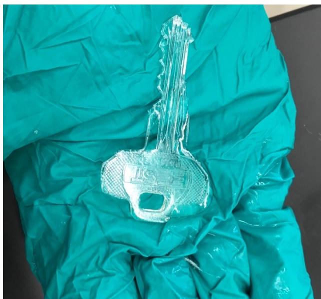
Figure 6. PVPON-PEGDA hydrogel replication of a key. The exact form of the key was retained by the PDMS mold, and the resulting clear hydrogel elastomer even retained the cross-hatching of the top section after photopolymerization.
