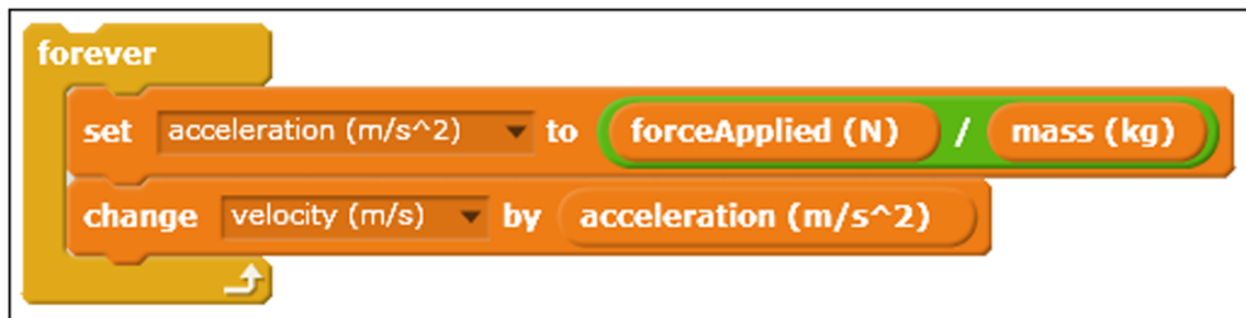
Fig. 6 Calculating velocity using block-based code
