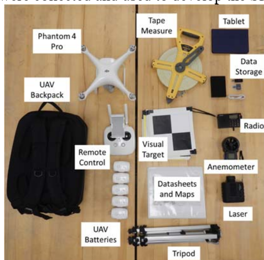
Figure 2. Equipment used for UAV-enabled SfM mapping in New Zealand (missing from the photo are the GNSS receivers used for ground control points).
