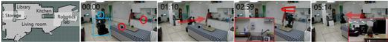
Fig. 4: Experiment with a language command “Find mugs in the kitchen and a book in the library”. The first image shows an occupancy grid map and semantic map of the environment. Red and blue circles indicate mugs and book respectively, and the blue box indicates the robot MOVO. The robot directly moves to the kitchen, looks around, and finds the first mug at 02:59. The inset images (red box) is the robot’s view. The second mug is found in the kitchen at 03:27, after 6 actions. The robot next moves to the library, looks around again, and then finds the book at 05:14 ( 3 additional actions).
