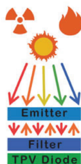
Figure 1. TPV system. Thermal energy from a heat source is absorbed by an emitter, which radiates infrared photons toward the TPV diode. Prior to the TPV diode stage, additional filtering may be incorporated. The radiation is then absorbed by the TPV diode, which generates a current and a voltage via the photovoltaic effect.
