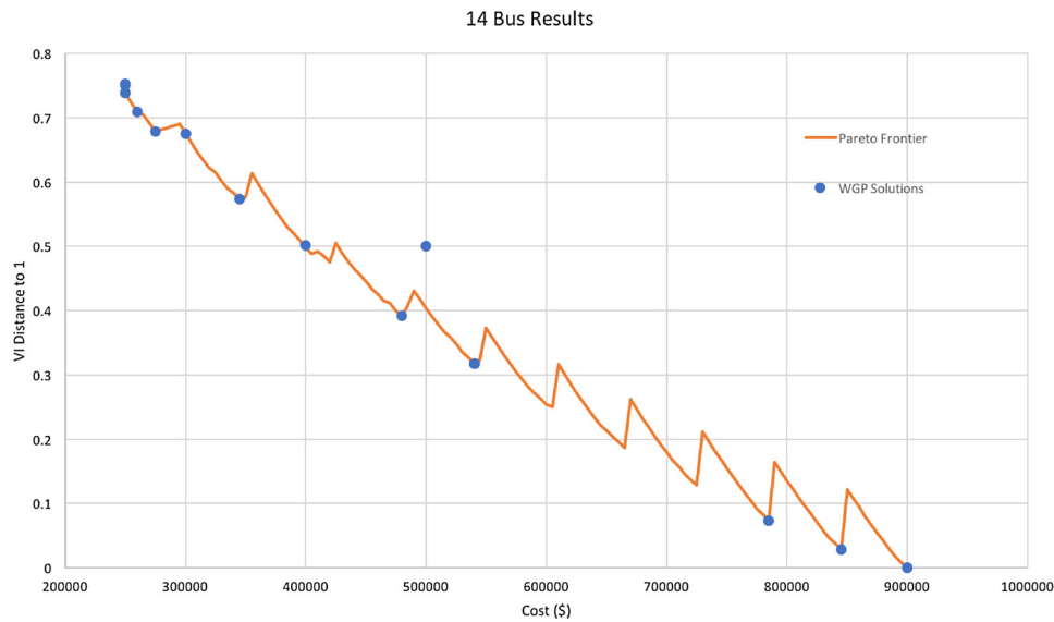
Fig. 3. 14 bus results of WGP framework along with Pareto frontier.
