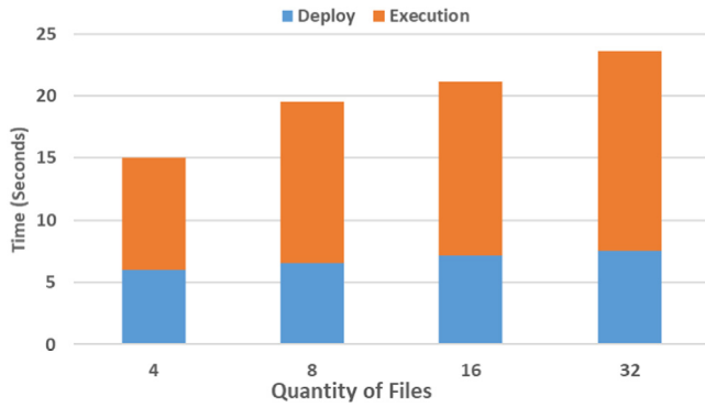
Fig. 6. The overhead of AM creation on WordCount by varying the number of files.
