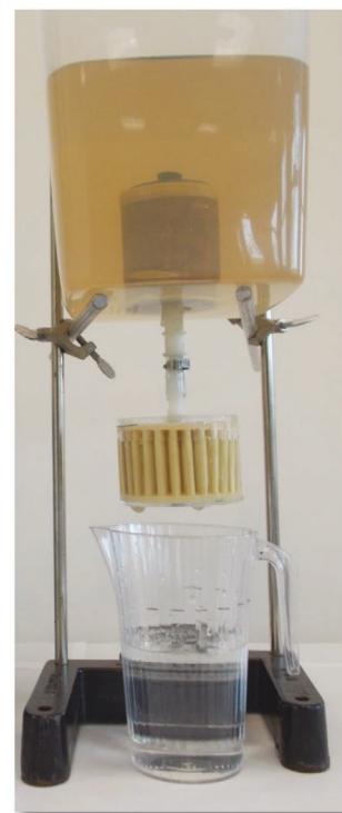
Figure 15. An experimental gravity-driven microfiltration unit with membrane (in the pleated format) having both filtration and adsorption capabilities.
