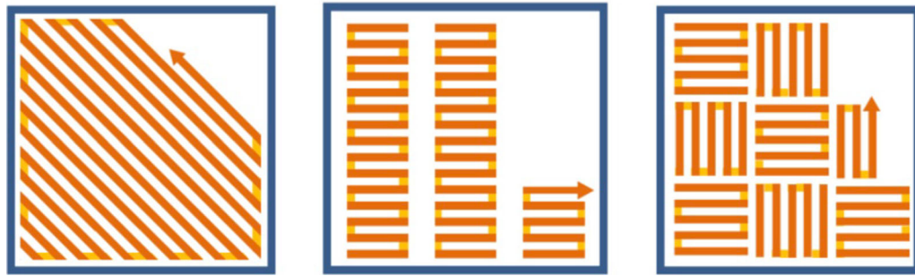
Fig. 1—Schematic illustration showing the laser scanning strategies used in the current study: (a) Meander, (b) Stripes, and (c) Chessboard (Reprinted with permission from Ref. 20).
