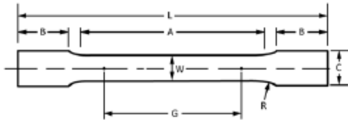
FIGURE 1: DEFINED DIMENSIONS BY ASTM E8 FOR A TENSION TEST SPECIMEN.
