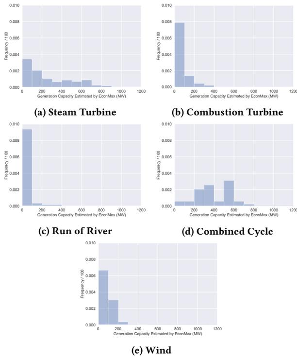
Figure 4: Distribution of Generation Capacity (MW) by Generation Type
