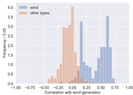
Figure 5: Distribution of Correlation Coefficient with Total Wind Generation by Generation Type
