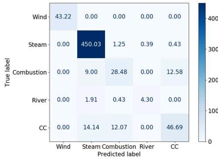
**Figure 9: Confusion Matrix for One-stage Random Forest Classifier, weighted by Power Generation (TWh)**
