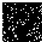
Fig. 4: Sample 33 \times 33 SBHE pattern (Hadamard block size = 16) used to simulate CS acquisition of RCM images.
