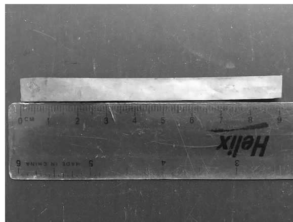
Fig. 1 Ionic polymer–metal composite used in experiments
