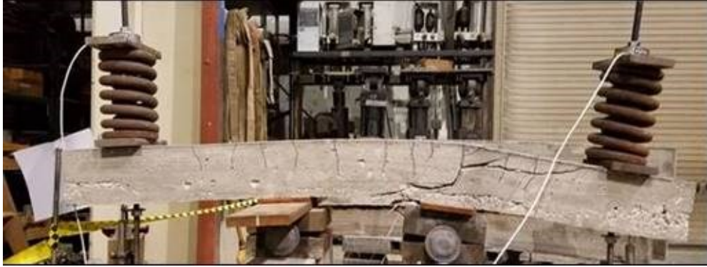
Figure 9. Failure of B-SL-81 (photo by S. Orton).
