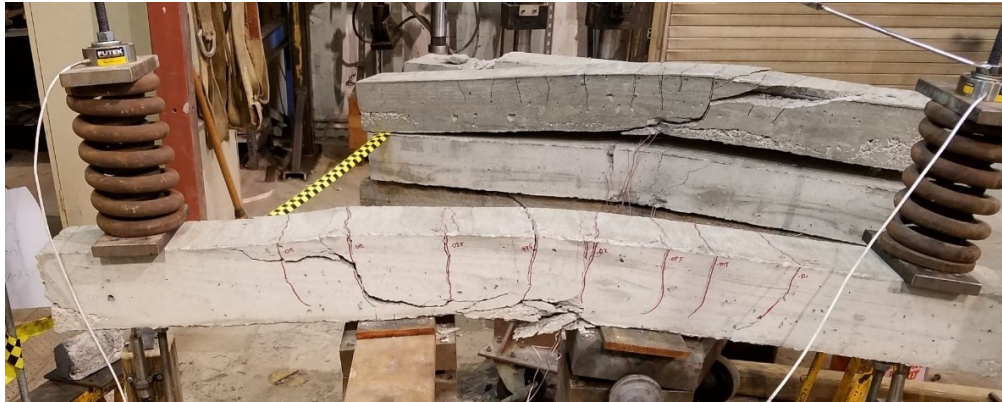
Figure 10. Failure of B-SL-86 (photo by S. Orton).
