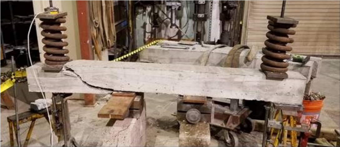
Figure 6. Shear failure mode of the control test (photo by S. Orton).
